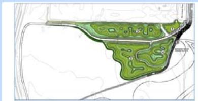
Figure 1. Letter A represents where the urban runoff enters into the treatment pond one. It is then diverted under a constructed berm by a culvert to direct flow into treatment pond two. It is then filtered through and underneath the trail through a culvert into treatment pond three, where it filters through again and under a berm through a culvert into treatment pond four where it is filtered for a fourth time before being released into the salt water marsh, letter B.
